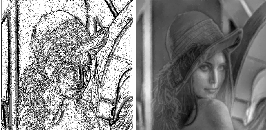
Figure 6: Left: Oriented MSM, from the MSM represented in Figure 4 . Black represents positive orientation, while gray means negative. Right: Reduced signal, generated by the only knowledge of the oriented MSM depicted on the left.
