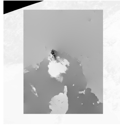
Fig. 4. Resulting multispectral reduced signal computed on a selected area of the original dataset. The plume only remains (with land pixels).
